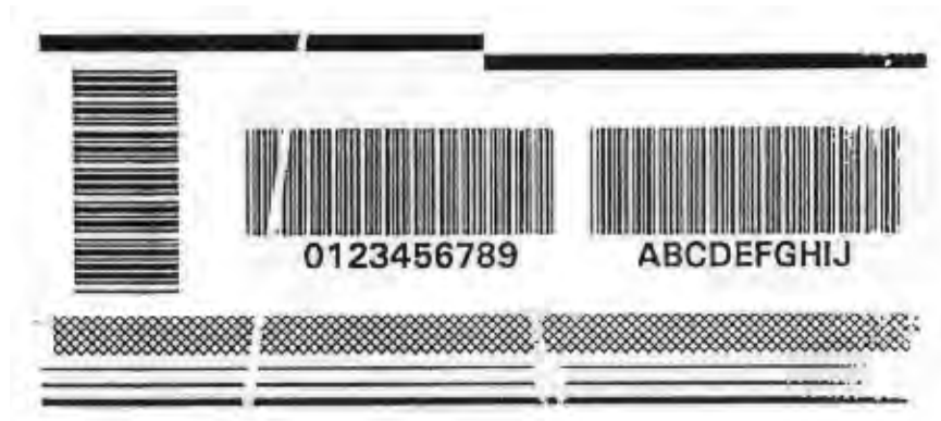
Figure 5-16 Sample of Ribbon Wrinkling
