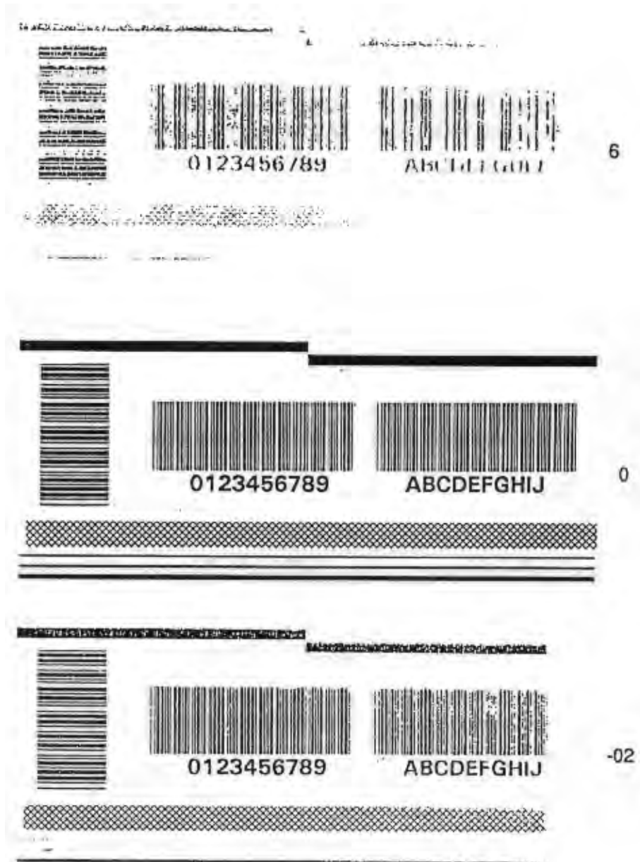
Figure 5-15 Samples of Incorrect Print Head Position Setting
